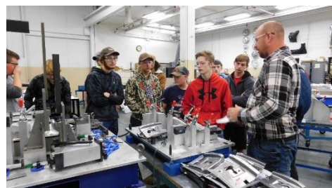
Tool & Die Designers, AJ Selleck (left) and Ted Murray (right) presented students with a look at a check fixture used for one of the many parts we are currently building dies for.
