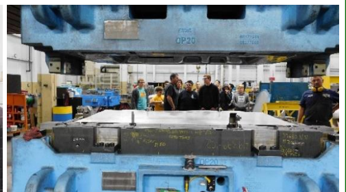
Tool & Die Maker, Jay Vlahas shows students how steel is formed using a die mounted in a press.
