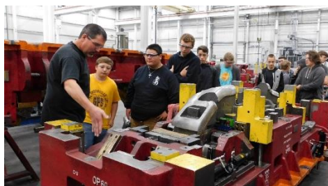
Tool & Die Maker, Ken Bradley explained to students how a die is used to make automotive parts.
