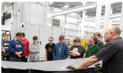
Tool & Die Makers, Joe Hoy (left) and Dave Bean (right) showed students how large sheets of steel are measured, cut and shaped to begin the tooling process.
