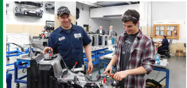
Tool & Die Maker, Kevin Lipp, showed Malachi a check fixture that is used to inspect the parts produced from one of the many dies we build. Thank you, Malachi, for your interest in tool and die making.
