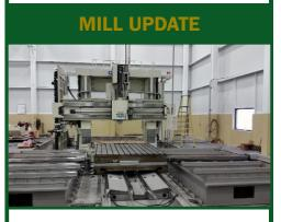
Installation of our new Okuma MCR-BII CNC bridge mill is almost complete. We are expecting the mill to be finished and in operation by the end of the month. This mill will greatly expand our capability to machine large steels and castings with an "X" travel of 196.9", "Y" travel of 145.7", and "Z" travel of 31.5".
